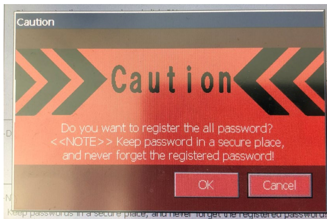
Figure 6. A typical message that appears when booting a robot for the first time, requesting the user to set a password, which is used to authenticate local operator access only
