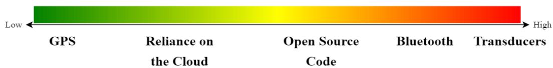
Figure 3. Common device capabilities ranked on level of risk they pose to the facility
