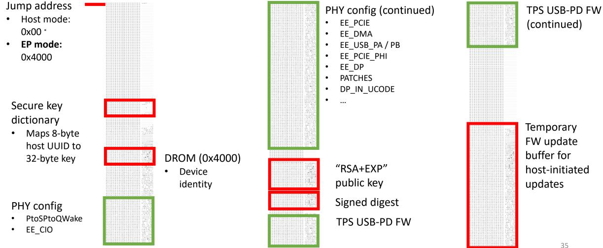
\*Offset varies by controller model, FW revision, and presence of secure key dictionary
