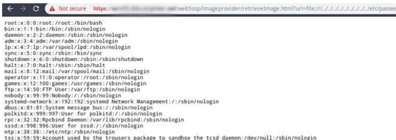
Figure: System file leaks
