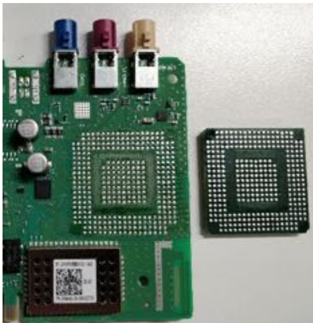
Figure: The LGA paddings of LTE module
