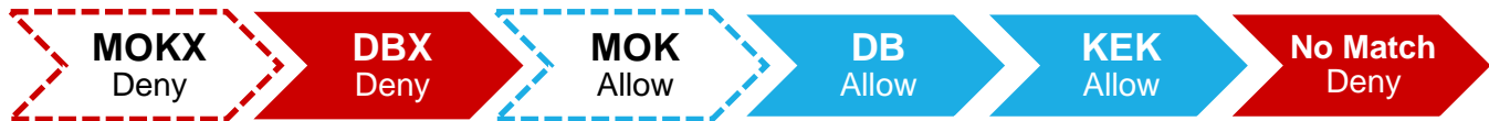
Figure 2 - Order of operations during UEFI Secure Boot checks. Checks contained within dashed lines only take place when the Shim bootloader is used AND after its initialization in the UEFI bootloader phase (i.e. firmware OROMs are not checked against MOKX and MOK; kernels are checked against MOKX and MOK).
