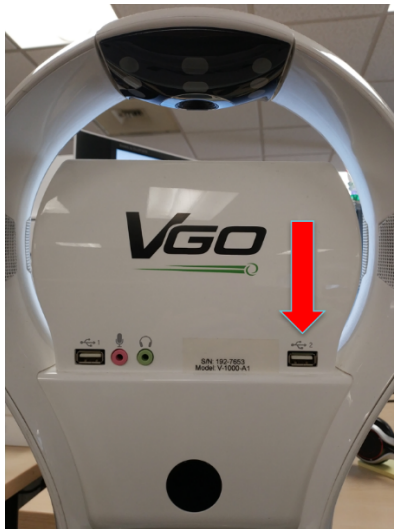
Figure 12: USB Slot 2 used for root access
