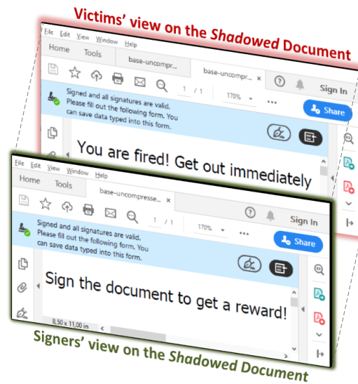
Figure 2.1: A signed PDF document remains valid after manipulations. A Shadowed PDF document presents a trustworthy content to the Signers . After signing the document, the attackers modify the document and enforce another view of the document on victims' side without invalidating the signature.
