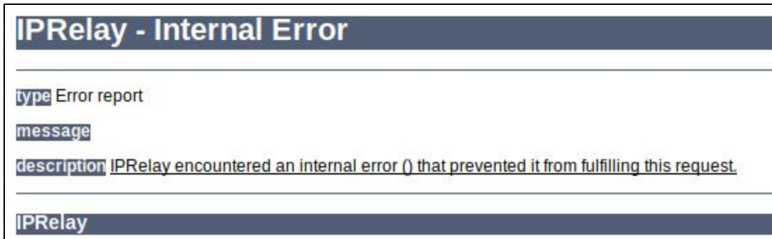
Figure 3: Response of https://<host>/IPRelayApp/servlet/IPRelay?page=../../../../../../../../etc/passwd?
