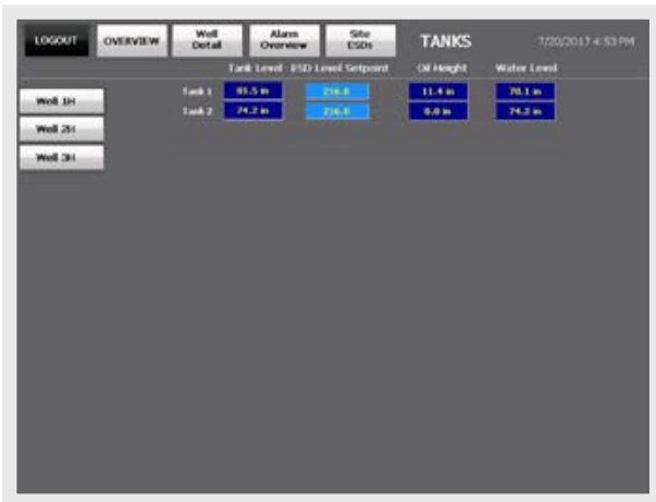
Page displaying oil and water levels in the storage tanks.
