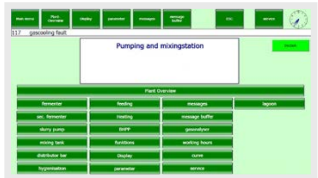
Top-level menu displaying the available submenus, such as Slurry Pump, Mixing Tank, Fermenter, Gasanalyser, Feeding, etc.
