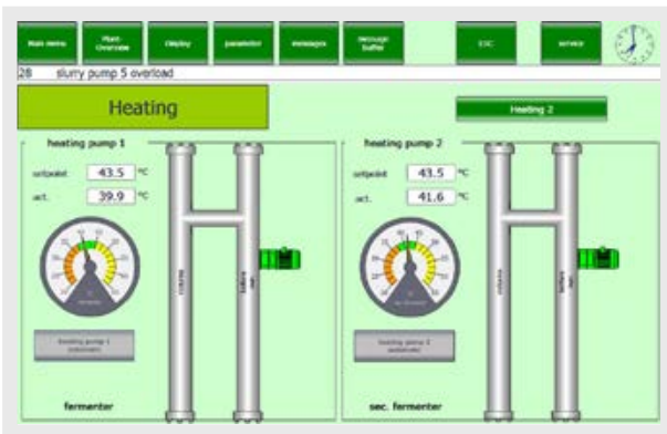
Heating controls. A “slurry pump overload” warning message is displayed at the top of the page.
