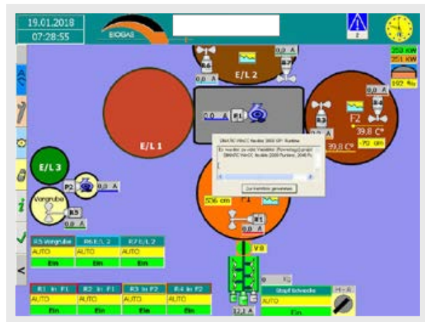
System in a German facility. The top-level menu has controls for pumps, air-gas mixers, circulation, start/stop, parameter adjustment, etc.
