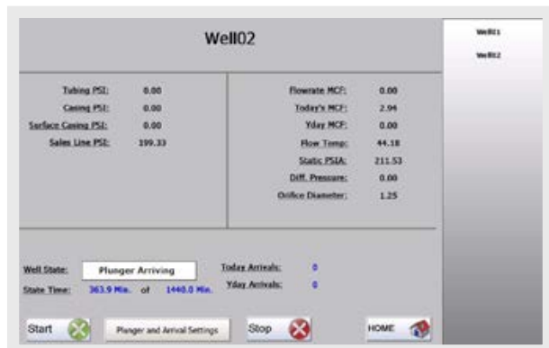
Displaying readings from a specific well. The start/stop controls and “Plunger and Arrival Settings” are accessed from this page.
