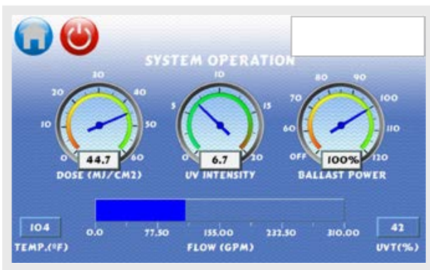
Water purification/disinfection plant in Canada. The page displays all subsystem status information in one screen. The HMI and/or system can likely be shut down from this screen.
