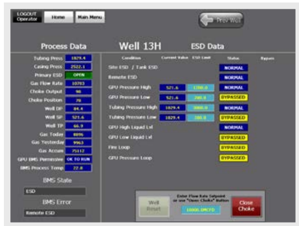
Individual well controls showing that a specific well can be either reset or “close-choked” (i.e., shut down) from this page.
