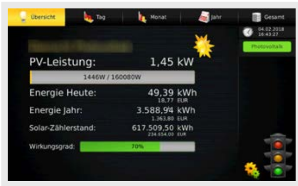
Main menu displaying energy generated by the solar cells.
