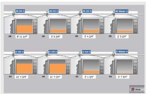
Display of storage tank oil and water levels.
