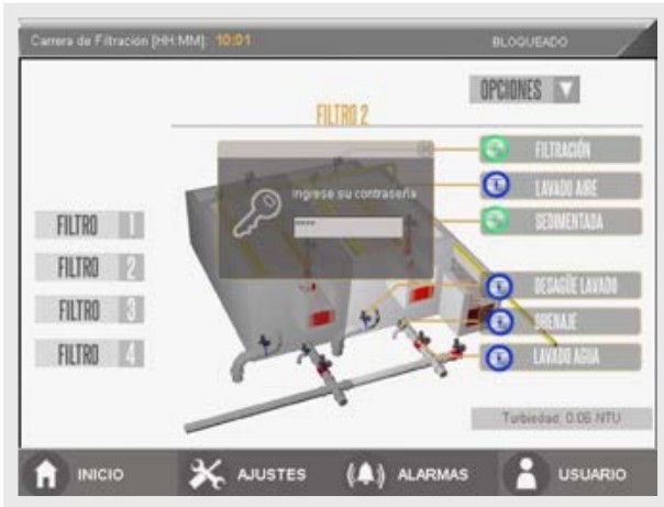
Water filtration facility in Colombia. The HMI requires user authentication before full menu access.
