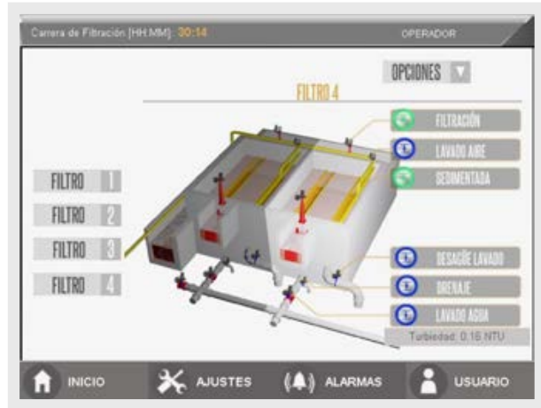
The same HMI without the user authentication pop-up window. It is unclear if the user has already authenticated, or if clicking on the menu items will bring up the user authentication window.
