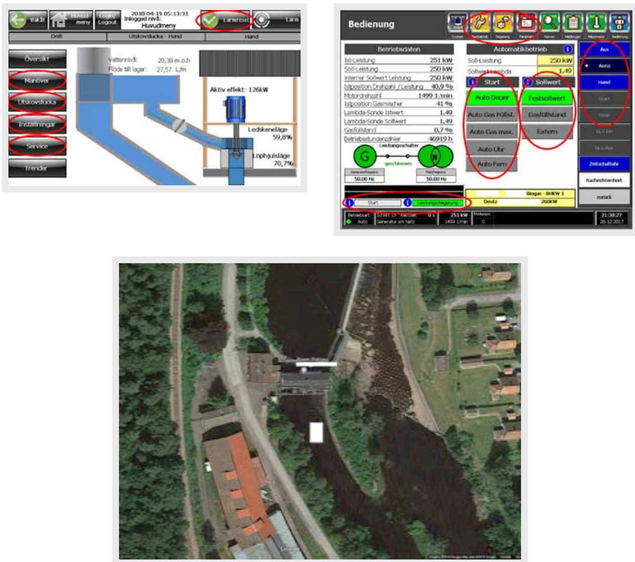
Figure 24. Screenshots of two exposed HMIs for control/configuration in power plants
